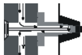
Conventional core cooling using a brass baffle.
